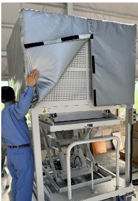
JacketFoam施工後 1300°C時外壁79°C
