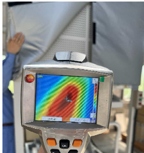
JacketFoam施工後 1300°C時外壁79°C
